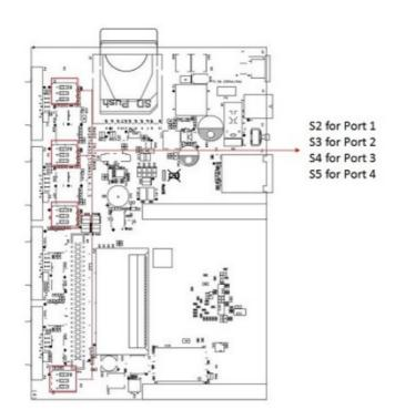
Dip switch Pin 1 and Pin 2 are used to set the pull up/down resistors. The default is 150 K $\Omega$ . Turn on dip switch Pin 1 and Pin 2 to set this value to 1 K $\Omega$ . Do not use the K $\Omega$  setting with RS-232 mode, since doing so will degrade the RS-232 signals and shorten the communication distance. Dip switch Pin 3 is used to set the terminator. Turn on dip
