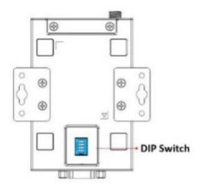
Open the back door with a screwdriver and use the DIP switch to set the pull high/low resistors. The default is 150 k $\Omega$ . You can switch the SW1 and SW2 to ON and change the value of the resistor to 1 k $\Omega$ .
