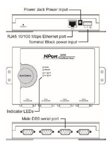
**Reset Button**—Press the Reset button continuously for 5 sec to load factory defaults: Use a pointed object, such as a straightened paper clip or toothpick, to press the reset button. This will cause the Ready LED to blink on and off. The factory defaults will be loaded once the Ready LED stops blinking (after about 5 seconds). At this point,
