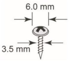
screws per bracket to attach the NPort 5400 to a wall or cabinet.
