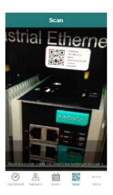
To view the status of a device on MXview ToGo, use the Scan page to scan the QR code on a Moxa device managed by the MXview server. The Device Status page is displayed.
