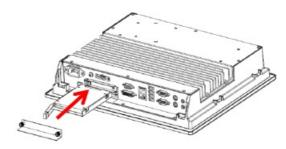
4. Reattach the HDD/SSD cover and fix it to the front panel with the 2 screws.
