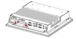
3. Insert the HDD/SSD (with the bracket) into the HDD/SDD slot. Noted that the latch on HDD/SSD bracket should be released when pushing the HDD/SSD into the slot.
