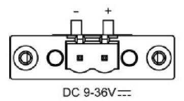
The MPC-2150 allows using either an AC or DC power input. When using AC power, use the standard C14 AC inlet. When using DC power, use at least a 60 W power adapter through the 2-pin terminal block in the accessories package. The figure shows the MPC-2150's DC pin assignments.
