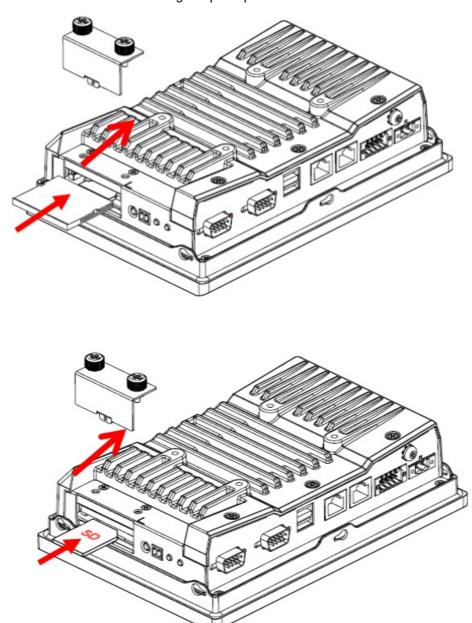
3. Reattach the cover and secure it with screws.
