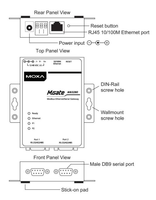
**Reset Button**—The reset button is used to load factory defaults. Use a pointed object such as a straightened paper clip to hold the reset button down for five seconds. Release the reset button when the Ready LED stops blinking in order to load the factory defaults.
