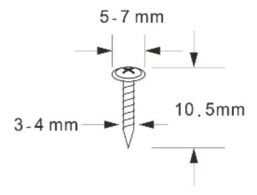
Mounting the MGate MB3180 onto a wall requires two screws. The head of the screws should be 5.0 to 7.0 mm in diameter, the shaft should be 3.0 to 4.0 mm in diameter, and the length of the screws should be at least 10.5 mm.
