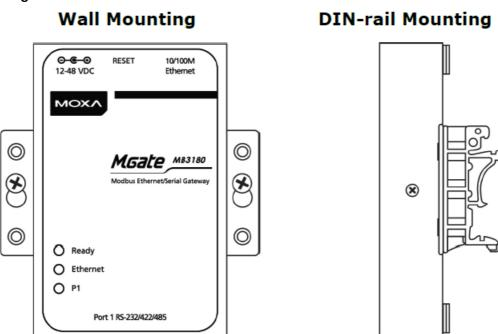
DIN rail attachments can be purchased separately to mount the MGate MB3180 on a DIN rail.
