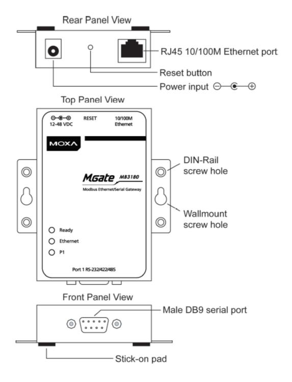
As shown in the following figures, the MGate MB3180 has one DB9 male port for transmitting serial data
