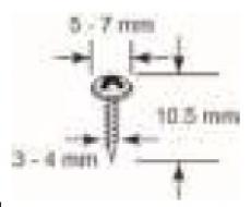
Mounting the MGate MB3170/3270 Series on to a wall requires two screws. The heads of the screws should be 5 to 7 mm in diameter, the shafts should be 3 to 4 mm in
