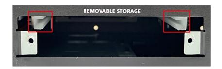
**Step 6:** Pull the latch on the tray to the right to secure the tray in the slot.
