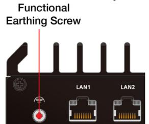
**NOTE:** A 4 mm2 conductor must be used when the connection to the external grounding screw is utilized. The heat sink is grounded to the chassis by an internal screw.
