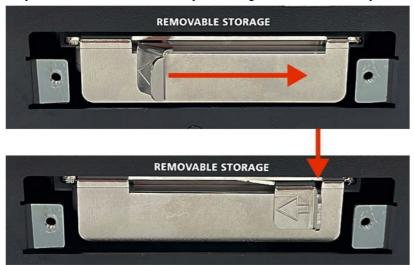
Step 7: Put back the cover on the storage slot and fasten the two screws to secure the cover in place.
