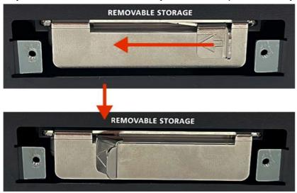
Step 3: Place the storage disk onto the tray.
