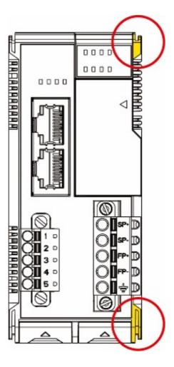
**Step 2:** Align the 45M module side by side with the head/CPU module and then push the 45M module until it touches the DIN rail.
