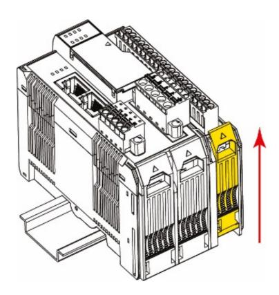
**Step 2:** Push the top of the release tab to latch it, and then pull the module out.
