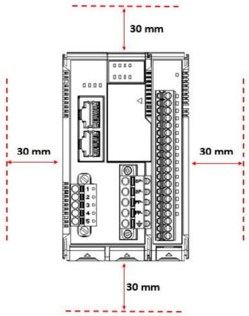
To ensure that the device works properly, we suggest reserving the amount of space indicated in the adjacent figure.
