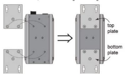
**STEP 2**: Mounting the EDS-G512E-8PoE series on the wall requires 4 screws. Use the EDS-G512E-8PoE series, with wall mount plates attached, as a guide to mark the correct locations of the 4 screws. The heads of the screws should be less than 6.0 mm in diameter, and the shafts should be less than 3.5 mm in diameter, as shown in the figure on at right.
