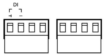
**STEP 1:** Insert the negative (ground)/positive DI wires into the  $\perp$ /I terminals, respectively.
