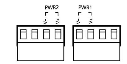
**STEP 1:** Insert the negative/positive DC wires into the V-/V+ terminals, respectively.
