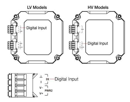
STEP 1: Insert the negative (ground)/positive DI wires into the \(\psi\_\)/I terminals, respectively.
