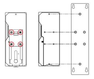
**STEP 2**—Mounting the EDS device on a wall requires six screws. Use the EDS device, with wall mount plates attached, as a guide to mark the correct locations of the six screws. The heads of thescrews should be less than 6.0 mm in diameter, and the shafts should be less than 3.5 mm in diameter, as shown in the figure on at right.
