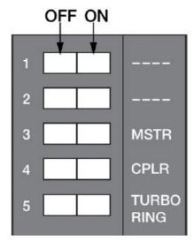
The default setting for each DIP Switch is OFF. The following table explains the effect of setting the DIP Switch to the ON position.
