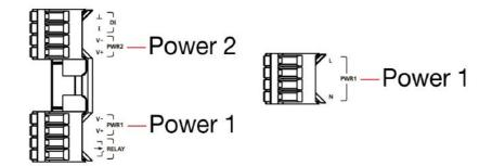
STEP 1: Insert the Positive/Negative DC or Line/Neutral AC wires into the V+/V- or L/N terminals, respectively.
