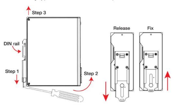
**NOTE** Our DIN rail kit now utilizes a quick release mechanism to make it easier for users to remove the DIN rail from the EDS device.
