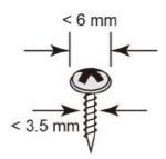
**NOTE** Before tightening the screws into the wall, make sure the screw head and shank size are suitable by inserting the screw through one of the keyhole-shaped apertures of the Wall Mounting
