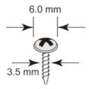
**NOTE:** Before tightening the screws into the wall, make sure the screw head and shank size are suitable by inserting the screw through one of the keyhole-shaped apertures of the wall mount plates.
