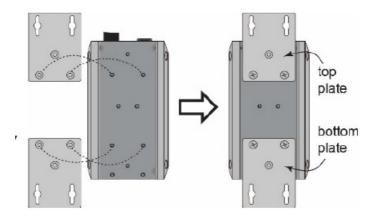
• STEP 2: Mounting the EDS-518E series on a wall requires 4 screws. Use the EDS-518E, with wall mount plates attached, as a guide to mark the correct locations of the 4 screws. The heads of the screws should be less than 6.0 mm in diameter, and the shafts should be less than 3.5 mm in diameter, as shown in the figure on at the right.
