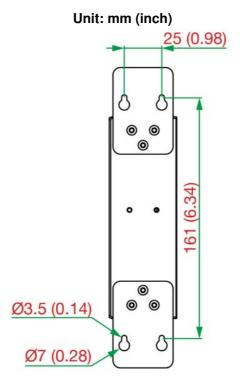
**STEP 2:** Mounting the EDR-G9004 Series on the wall requires four screws. Use the EDR-G9004 Series with the wall mount plates attached as a guide to mark the correct location of the four screws. The head of the screws should be less than 7.0 mm in diameter, and the shaft should be less than 3.5 mm in diameter.
