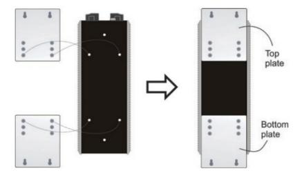
**STEP 2**—Mounting the EDR-810 on the wall requires four screws. Use the EDR-810, with wall mount plates attached, as a guide to mark the correct locations of the 4 screws. The heads of the screws should be less than 6.0 mm in diameter, and the shafts should be less than 3.5 mm in diameter, as shown in the figure on the right.
