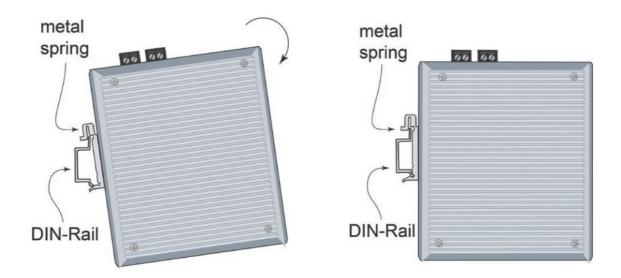
To remove the Industrial Secure Router from the DIN rail, simply reverse Steps 1 and 2 above.
