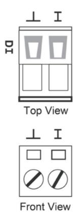
**STEP 1:** Insert the negative (ground)/positive DI wires into the  $\perp$ /I terminals, respectively.
