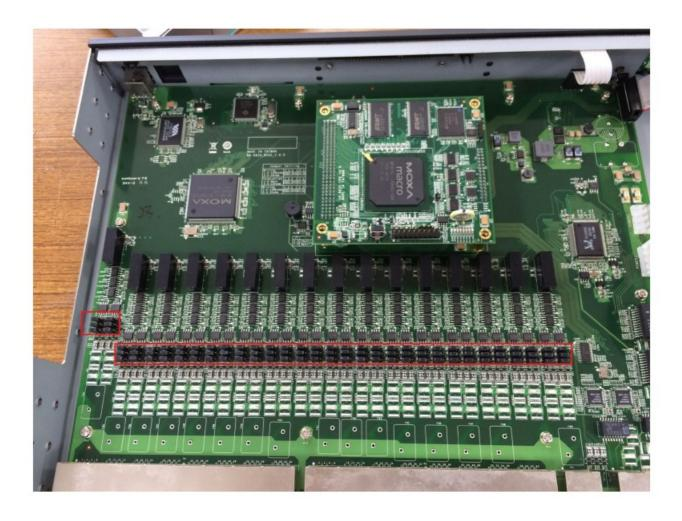
In some critical environments, you may need to add termination resistors to prevent the reflection of serial signals. When using termination resistors, it is important to set the pull high/low resistors correctly so that the electrical signal is not corrupted. The DA-660A uses jumper settings to set the termination resistors and pull high/low resistor values for each serial port.
