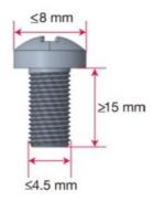
After mounting the BXP computer using the wall-mounting kit and fastening the 4 screws to fix the
