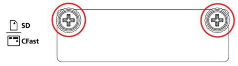
2. Remove the cover and locate the SD and CFast card slots.
