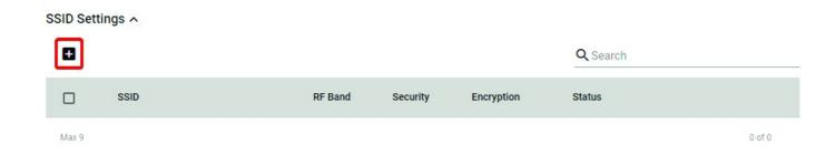
On the settings page, configure the SSID Status, SSID, RF Band, RTS/CTS Threshold, and Transmission Rate for the 5 GHz or 2.4 GHz band. When finished, click NEXT.
