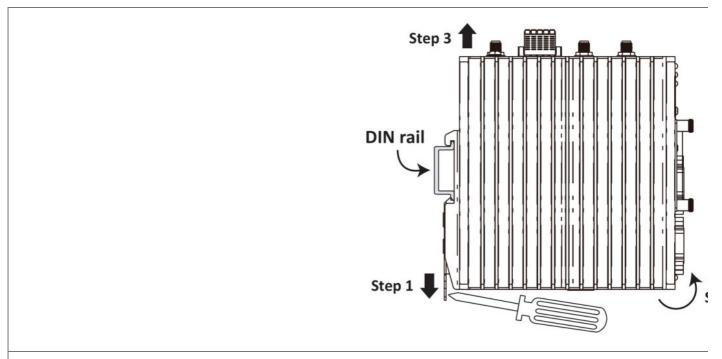
**STEP 1:** To unmount the AIG-500, pull down the latch provided at the base of the mounting kit with a screwdriver. STEPS 2 & 3: Slightly pull the AIG-500 forward and lift it up to detach it from the DIN rail.
