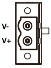
Connect the power jack (in the package) to the DC terminal block (located on the top panel), and then connect the pup. Once the system is ready, the power LEDs will light up.
