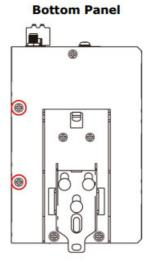
1. Loosen the six screws on the right panel and two screws on the bottom panel of your computer.
