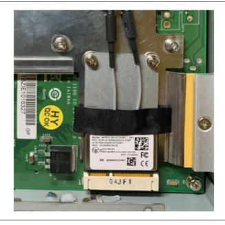
9. Stick a piece of insulation tape on the connectors as indicated.
