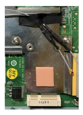
3. Remove the plastic sheet on the thermal pad and stick the thermal pad as indicated.
