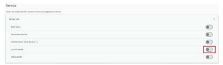
Security Check Criteria: Serial Console Service should not be We recommend disabling Serial Console Service
