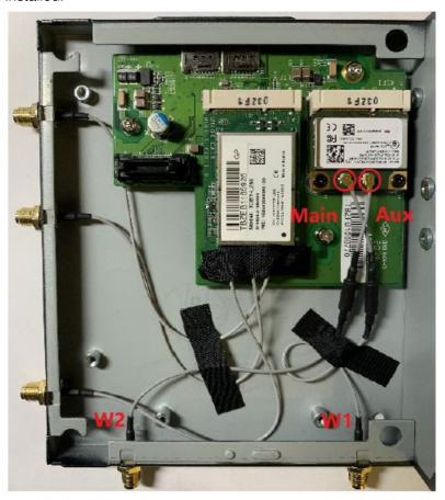
8. Stick the insulation tape on the connectors.
