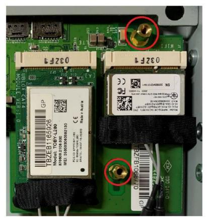
11. Remove the plastic sheet on the thermal pad of the heat sink, install the heat sink pad on the module, and secure the heat sink with the two silver screws (M3 x 6 mm).
