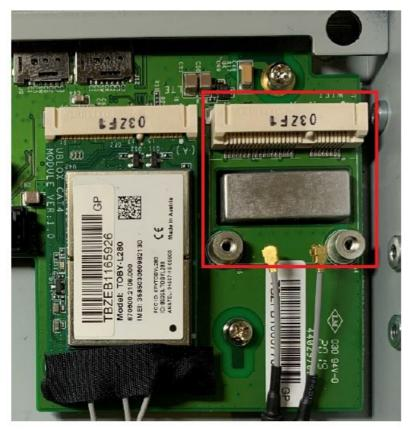
3. Remove the plastic sheet on the thermal pad and stick the thermal pad on the metal surface as indicated.
