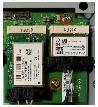
10. Fasten the two bronze screws on to the screws on the board.
