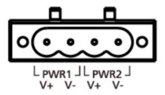
Use wires with 12 to 26 AWG wire size to connect to V+, V-, and GND.
