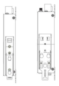
3. Latch the unit firmly on to the DIN rail as shown in the illustrations below.
