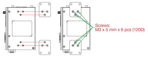
2. Use two screws to mount the AIG-100 on to a wall. These two screws are not included in the wall-mounting kit and must be purchased separately. Refer to the detailed specifications below:
