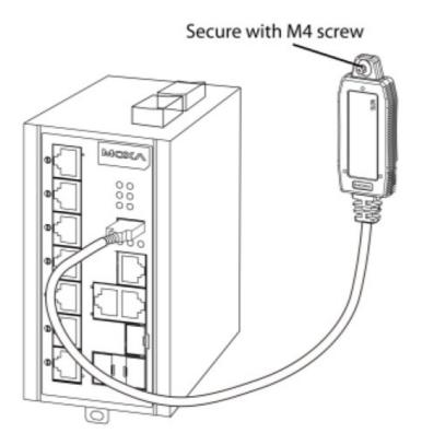
• Avoid hanging the ABC-02 configurator from the switch without securing it onto the wall.
