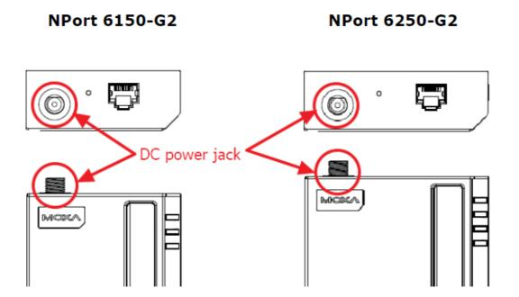
If you are connecting the DC outlet to a DIN-rail power supply, you will need a separate power cable, CBL-PJ21NOPEN-BK-30 w/Nut, to convert the terminal block output to the DC outlet on the NPort.
