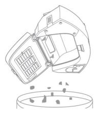
3. Remove the filters and tap the HEPA filter gently.
