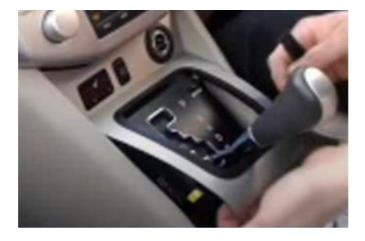
Step 2: Remove the Panel Underneath the Radio (unclip)
