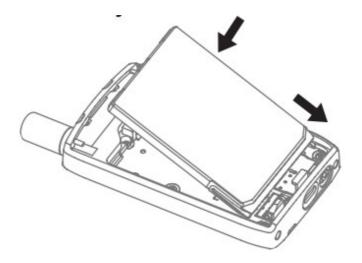
Insert the bottom part of the battery into the compartment. Press down the top part of the battery into the compartment until it clicks.
