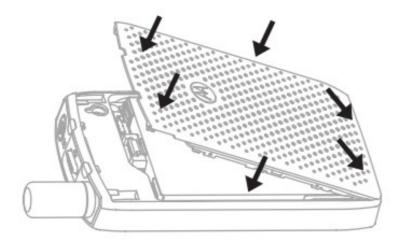
**To Attach:** Insert the bottom part of the battery cover into the slot. Press down the middle part followed by the top part of the battery cover until it clicks.
