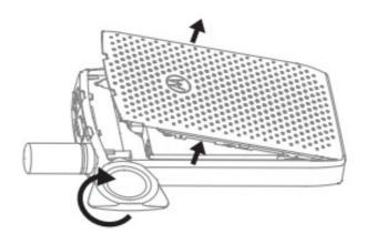
**To Remove:** Place and twist the battery cover opener at both top corner slots, one after the other. Lift up the battery cover along the side surface.
