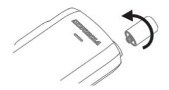
Turn the radio off before attaching the antenna. Align the bottom part of the antenna to the threaded base on top of the radio. Turn clockwise until snug. Do not force.
