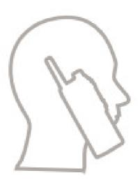
When making simplex calls (high audio), hold the radio in a vertical position with the top microphone 5 to 10 centimeters away from your mouth. Speak into the top microphone. Listen via the radio internal speaker. Keep the antenna at least 2.5 centimeters from your head and body.
