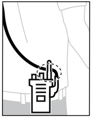
To ensure optimum range and user experience, it is recommended to avoid crossing accessory cable with the radio antenna.
