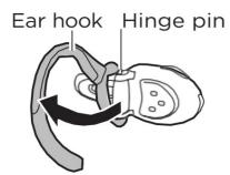
Open the boom and ear hooks and gently lift-top of the ear hook up and off, flip the headset over, and then hook the bottom of the ear hook onto the lower hinge pin and lift-top of the ear hook up and onto the upper hinge pin.
