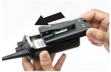
2. Flip the battery latch close and press it onto the battery until it locks in place.
