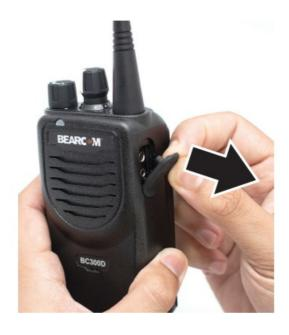
Postrequisites: Replace the dust cover when the universal connector is not in use.
