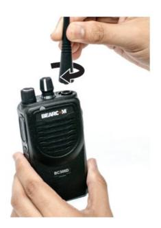
NOTE: Fastening the antenna blocks water and dust from entering the radio.
