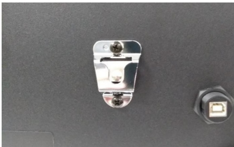
Figure 8: Installation of the Microphone Clip
