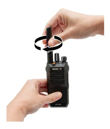
**NOTE:** Fastening the antenna blocks water and dust from entering the radio.
