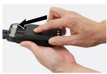
Press the battery firmly and slide upwards till the latch snaps into place..
