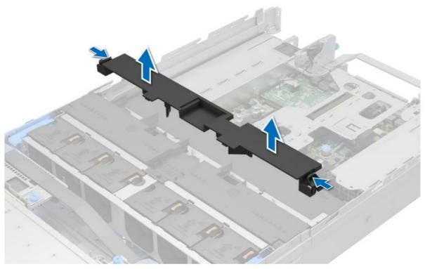
3. Hold and lift the filler from the GPU air shroud.
