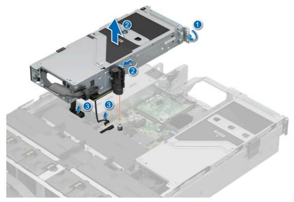
5. Lift the expansion card latch and remove the GPU blank from slots 7 and 8.
