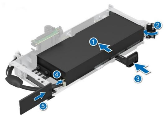
7. Reinstall the PCI riser cage back into the AI NVR 2 Premium Form D and reconnect any internal cables from the expansion boards.
