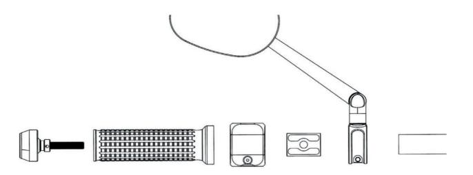
Drill 3 holes with 5mm diameter into the handlebar. Deburr the holes inside and outside carefully
