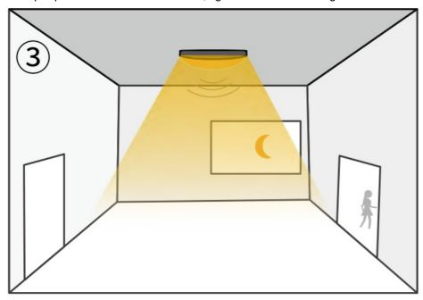
4. After the last detection and the preset hold time elapsed, light OFF.
