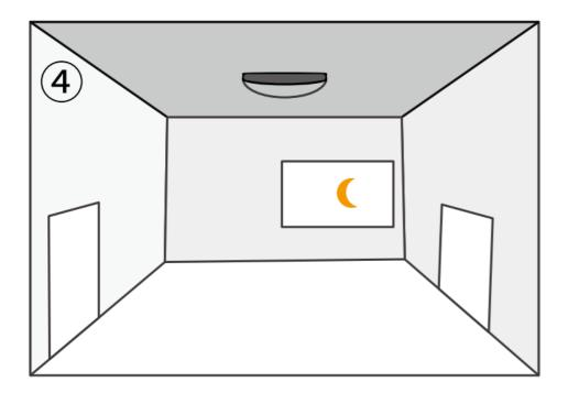
The daylight threshold is set to "Disable". Light on when detect movement, After people leave, Light off after Hold-time.
