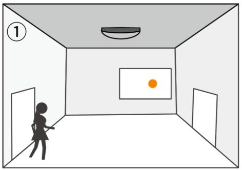
2. With insufficient daylight, when motion detected, light ON
