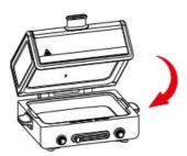
• The upper heating element will NOT work when the BASE HEAT function is selected, so the lid protection mechanism is not activated during the BASE HEAT function.
