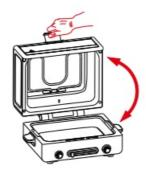
• Hold the door handle of the glass door and pull down and the glass door can be opened to an angle of 90°-95°.
