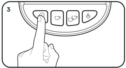
When the One Cup and Two Cup Buttons (2/3) illuminate solidly, place the Steam Wand (12) into a mug or jug and slowly turn the Steam Control Dial (6) until the water dispenses – keep the Dial open for at least 30 seconds and close the Dial. Take care performing this process as the hot water will pulse into the receptacle, and it may emit steam. Dispose of the water and repeat the process a further two times.
