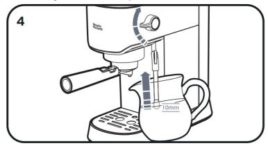
Press the Steam Button (4) to exit the steam function. Serve the frothy milk. Press the On/Standby Button (1) to turn off the unit.
