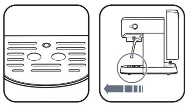
When the water in the Removable Drip Tray (14) is full, the Drip Tray Full Indicator (15) will be visible.
