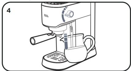
Following action no.4, wait for the One Cup and Two Cup Buttons (2/3) to illuminate solidly. Then place a receptacle, capable of holding 150ml, on the Drip Tray Grid (11) and press the Two Cup Button (3).
