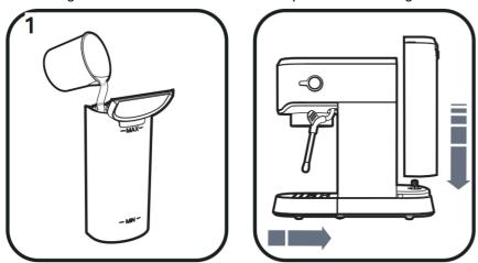
Fill the Water Tank (8) up to the MAX line. Assemble the Espresso Coffee Machine as above, ensuring the Removable Drip Tray (15) is in place.
