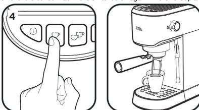
When the One Cup and Two Cup Buttons (2/3) illuminate solidly, place your cup(s) on the Drip Tray Grid (11). Press either the One or Two Cup Button to dispense set amount, approximately 50ml for one cup and 100ml for two.
