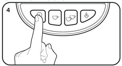
When the One Cup and Two Cup buttons (2/3) stop pulsing, place your cup(s) on the Drip Tray. Press either the One or Two Cup Button to dispense the set amount: approximately 40ml for one cup and 80ml for two. At the end of the dispensing time, the machine will beep once.
