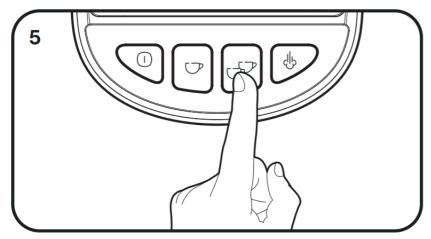
Water will pass through the system into the receptacle, which then must be emptied. Repeat a further 3 times – the coffee machine is now primed for making coffee.
