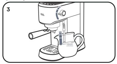
When enough froth has been produced, turn the Steam Control Dial (6) to OFF.
