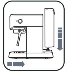
Without placing any Filters (17/18) into the Filter Holder (19), place the Filter Holder into the Brewing Head (10) and turn until at a right angle to the Main Unit to lock into position securely.
