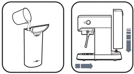
Fill the Water Tank (8) up to the MAX line. Assemble the Espresso Coffee Machine as above.
