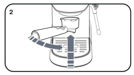
Place the Coffee Filter (17/18) into the Filter Holder (19) without coffee in the Filter. Place the Filter Holder into the Brewing Head (10) and turn until at a right angle to the Main Unit to lock into position securely
