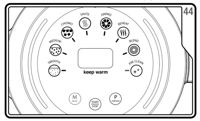
• 45 Press the Start/Stop Button (23) and the processing time will count down on the LED screen (21). The Pre-Clean program will run for 4 minutes.
