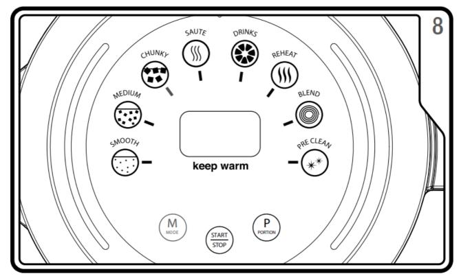
• 9 Press the Start/Stop Button (23) and the processing time will countdown on the LED screen (21). Portion control is set to 2 portions. If 3 or 4 portions are required it must be set before the Start/Stop Button (23) is pressed. See portion control on page 8. Smooth and drinks function will be set to 3 portions.
