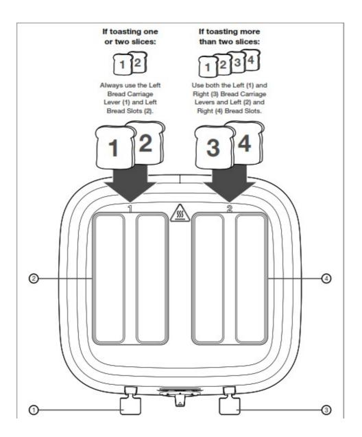
The Right Bread Carriage Lever (3) will not operate unless the Left Bread Carriage Lever (1) is in use.
