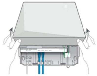
**Step 3**Ensure that the power cable is securely in place and that the Power and Optical lights are showing as steady green on the nbn® Connection Box.
