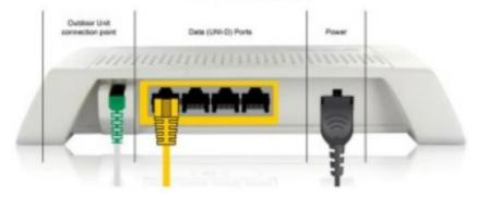
Using an ethernet network cable connect your router from its WAN port to the relevant Uni-D port on the NBN Connection Box. We generally activate the next available Uni-D port starting with Uni-D 1. We will detail your Uni-D port number in our emails to you.
