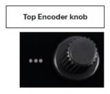
• FOR EXAMPLE – If you have a vocal mic plugged into Input #1 on the HUB, you first select channel 1 with the top encoder. You then use the bottom encoder knob to set the gain of the selected Input. The bank of buttons to the left of the HUB screen can be used to select other preamp options. These include: 48V (phantom power), PHASE (reverse), HI PASS (filter for cutting low frequencies), DIRECT (monitor direct input or effected signal from DAW), and INST (for unbalanced instrument inputs).
