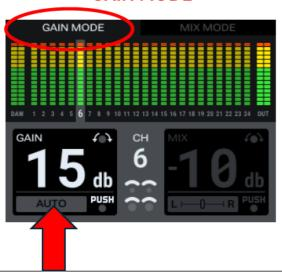
IMPORTANT: Note that while you are in GAIN MODE, the LOWER LEFT SIDE of the screen is ACTIVE.
