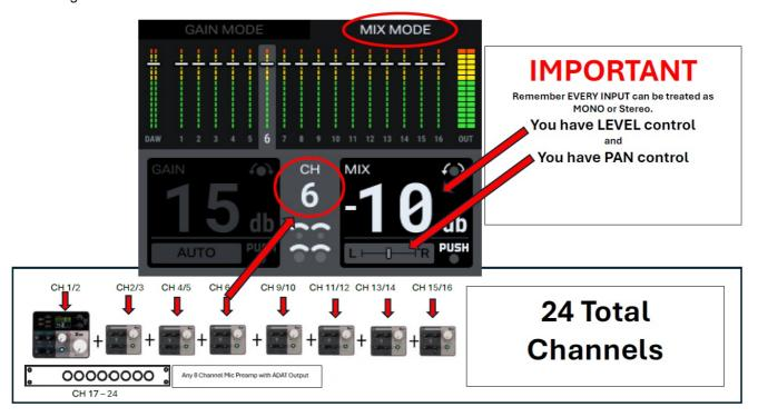
All inputs that plug into a local HUB or 2X/4X/8X unit are always available on the local box MIX knobs.
