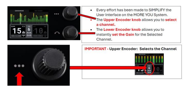
The 3 dots indicate moving to a Channel
