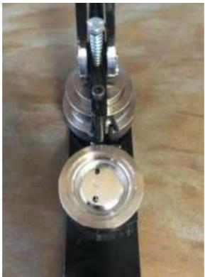
Rotate dies counterclockwise so that the pin back is under the upper die. Pull down the red handle.
