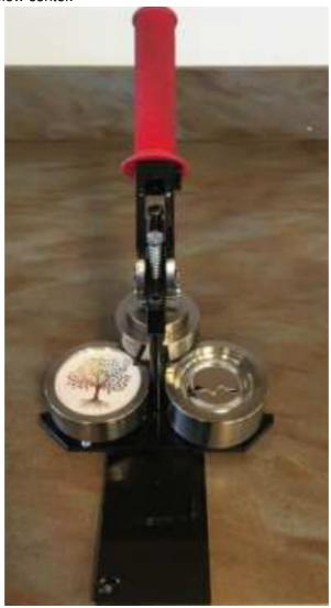
Rotate the left die clockwise. Pull down the red handle. Use your muscles! The components will be picked up and stay in the upper die.
