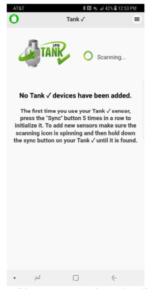
3. Press and hold the SYNC button until the sensor appears on the app. (up to 10 seconds)
