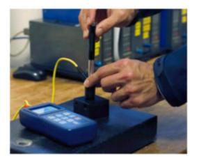
• Push down the sleeve to 'load' the probe and prepare for testing.
