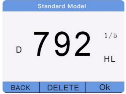
Measure 5 points vertically downward on the calibrated Leeb hardness block. After measuring 5 points, the display will show the average value and AVE sign.
