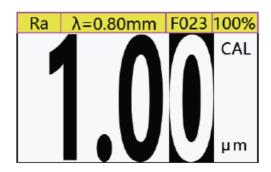
• After calibrating the measured values, press the key for 3 seconds to save the calibration and exit the CAL indicator on the screen will disappear.
