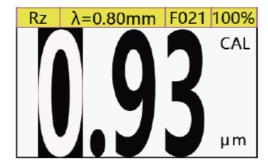
• When entering the calibration mode, press the button to adjust the display value to the digit that needs to be modified, and press the or button to adjust the value to the correct roughness for the measured sample. The nominal value of this sample is 1.00, as shown in the following figure.
