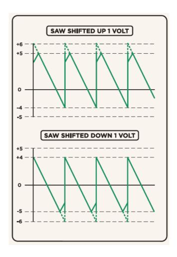
However, if we shift the entire wave up or down, the wave folder will now distort the top and bottom of the waves differently.
