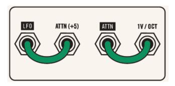
With the attenuator knob fully clockwise you will hear the same 10-octave trill, but as you lower the attenuator knob that range will diminish until there is almost no modulation.
