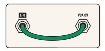
Now you can hear the volume move up and down in time with the LFO—even when no key is pressed. This is because now the LFO signal is controlling the volume instead of the envelope generator. By turning the filter CUTOFF knob completely counterclockwise we can then silence Mavis when no key is pressed.
