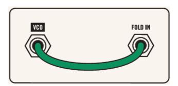
Open the VCF CUTOFF knob fully clockwise so you can hear the folding more clearly. Now by rotating the FOLD knob you will hear the oscillator begin to distort and fold over on itself. Try changing the VCO WAVE between saw and square and listening to how that affects the FOLD. You'll notice using a square wave that the wave folding has a much more subtle effect.
