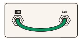
Now the LFO is connected to the GATE triggering a new note with each LFO pulse via a patch cable, and the LFO is also connected to the S+H GATE through normalization. Now you will hear a procession of distinct random notes. Remembering back to our first patch, you will probably note that, again, the range of notes is quite wide—far too wide for some musical purposes.
