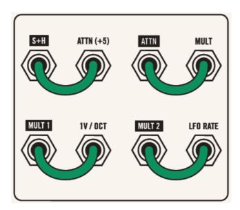
The MULT is a simple utility allowing you to patch one output to multiple inputs. Patch the S+H output (post attenuator) to the MULT input, and then patch MULT 1 to the 1V/OCT and MULT 2 to the LFO RATE.
