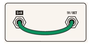
You will hear a new pitch in time with the LFO. If the VCO WAVE knob is rotated to the square wave you will hear only two pitches since the square wave being sampled only oscillates between two voltages. If the VCO WAVE knob is turned to sawtooth you will hear random voltages, as the sawtooth wave sweeps continuously between +5 and -5 volts and (typically) at a rate much faster than the LFO.
